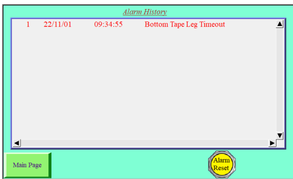
Figure 70: HMI Alarm Screen
