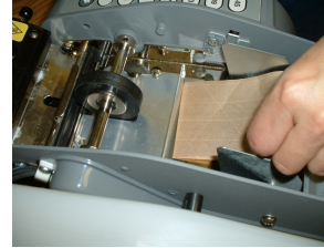
Feed tape under upper plate
