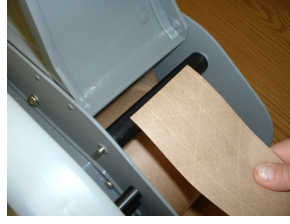
Feed tape over roller
